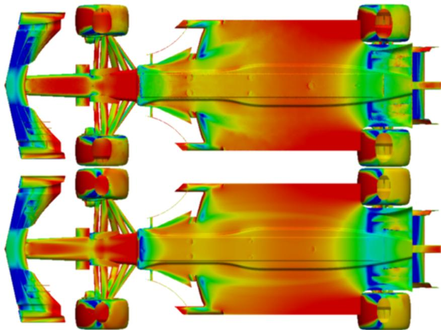
CD and CL within 4% . 20x more cells in Fluent mesh.
